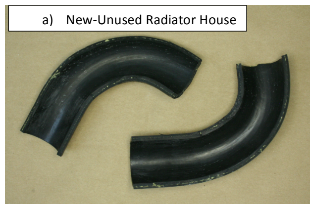
Fig 7. Radiator Hoses that have been cut open to expose the interior surface: a) New Unused Radiator Hose b) Prestone Cor-Guard, from Vehicle 304 after 80K miles c) Factory Fill, from Vehicle 312 after 80K miles.
